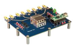
The 050-338-EVALBOARD can be used to evaluate PCB Mount Quad Optical Transmitters and PCB Mount Quad Optical Receivers. The evaluation board has been designed for high data rate operation and incorporates 8 SMA connectors that interface with high speed 100 ohm differential lines which can support testing of products up to 10Gbps data rates.
