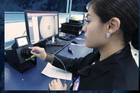
**Inspection and Test** Each and every fiber optic circuit is 100% polished, cleaned, and inspected prior to shipment.
