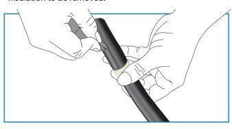
C) Using needle nose pliers, grab the insulation material where the lenghtwise score meets the guide mark. Gently pull the insulation away, working downwards along the incision towards the end of the cable. Once insulation is removed wire is ready for crimp termination.
