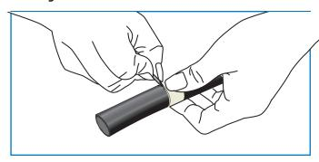
**B)** Score insulation lengthwise along the entire section of insulation to be removed.
