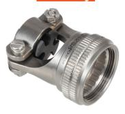
620PS076 heavy-duty clamp fits Glenair Series 970 PowerTrip® connectors. Anti-decoupling mechanism provides audible detented coupling and prevents backoff under high vibration. Saddles have self-locking stainless steel clinch nuts. Rigid dielectric bushing provides additional wire support (not available for all insert patterns). Full radius saddles are intended to be fully closed (bottomed onto frame).
