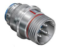
970-005 cable-mount receptacle has accessory thread for attaching strain relief clamps, backshells or adapters. Coupling threads are triple-start ACME quick-disconnect. EMI protected with ground spring on plug. Aluminum or stainless steel shell has five polarizing keyways. Crimp rear-release contacts are packaged with connector. PowerTrip connectors feature low resistance LouverBand contacts and are designed to withstand extreme environments.
