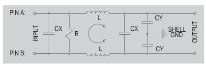
modern filter elements incorporating compensating inductors or coupled chokes. PowerTrip powerline filters are typically supplied as made-to-order (bespoke) solutions. Please contact the factory for application engineering assistance.
