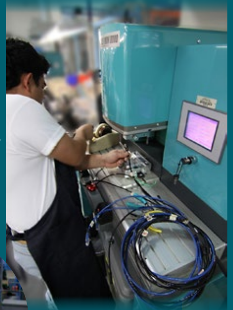
Precision overmolding of harsh environment connector assemblies with chemically-resistant materials such as Viton® and Duralectric®
