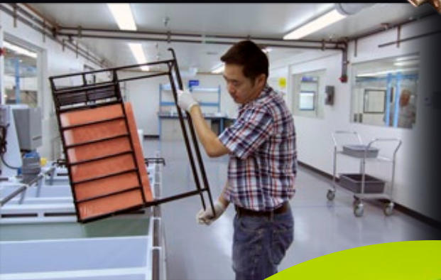
Panel preparation, chemical wash, etching and plating
