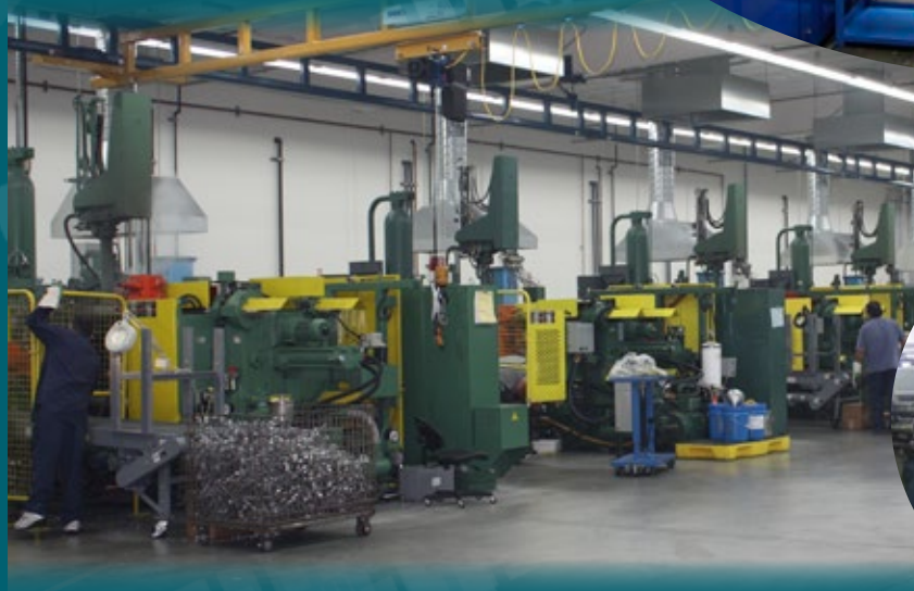
Glenair's die casting operation supports large-volume interconnect requirements—from backshells to conduit fittings, industrial connector shells and more
