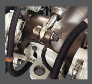
Turnkey wheel well impact-resistant metal-core conduit assembly Metal-core conduit wire protection aircraft brake assembly Brass, SST, or nickel-iron metalcore conduit material types with innovative microfilament and drawn filament braiding. Factory terminated or for use with userinstallable fittings.
