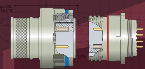
Circular connector coupling technology: the ubiquitous MIL-DTL-38999 Series III circular features one of the most popular connector coupling designs, the triple-start stub ACME thread. In addition to fast and reliable mating, this threaded coupling design has the advantage of a ratcheting anti-decoupling mechanism, receptacle striping indicating full mating, and metal-to-metal bottoming between the mating pairs for reduced electrical resistance.
