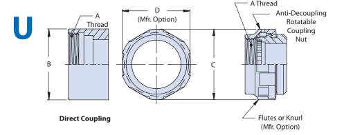
Note: Direct coupling supplied with O-ring for moisture sealing. Add modifier code 101A to end of part number for O-ring to be supplied on rotatable coupling.
