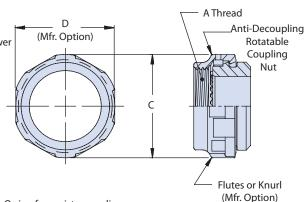
Note: Direct coupling supplied with O-ring for moisture sealing. Add modifier code 101A to end of part number for O-ring to be supplied on rotatable coupling.
