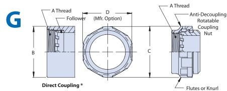
Note: Code G, rotatable coupling is supplied without O-ring. Environmental seal performed by interface geometry.
