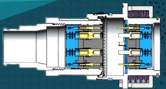
Figure 1: Key and keyway engagement ensures polarized mating and axial alignment
