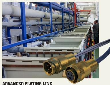
Capabilities include VG95328-qualified Marine Bronze and "Code J" Tin-Zinc plating—VG95211 and VG95212 qualified cadmium alternative for corrosion-resistant interconnects.
