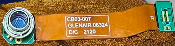
Point-to-point rigid-flex assembly for a downhole tool application
