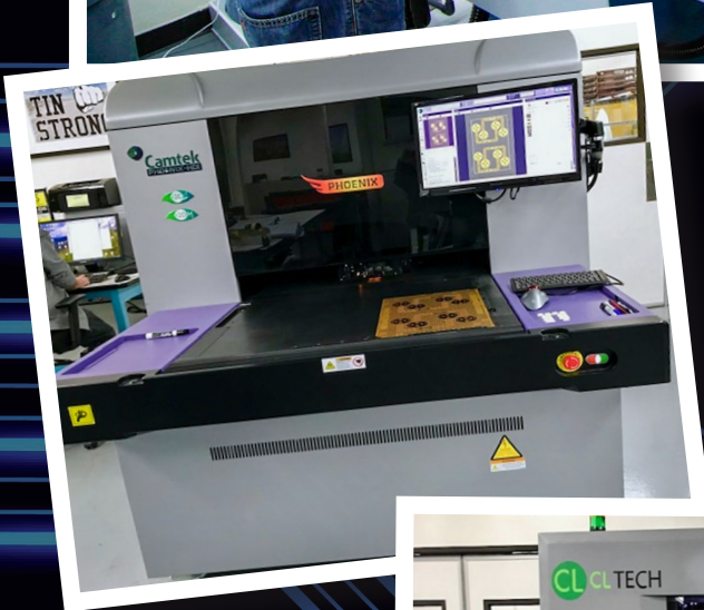
Automated Optical Inspection and Flying Probe Electrical Test
