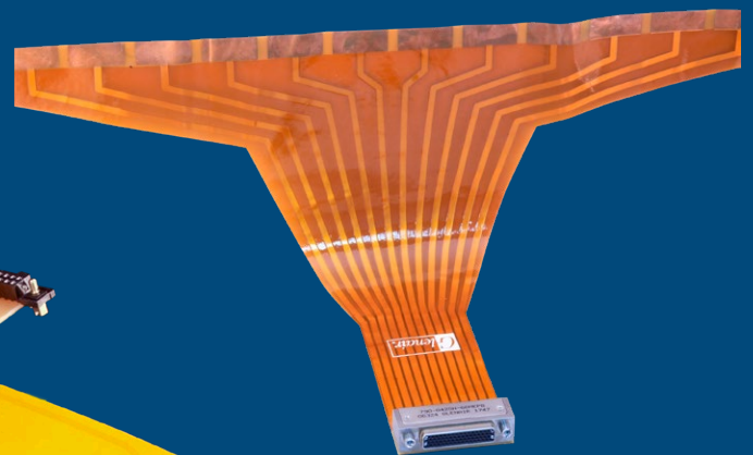
Flex assembly with Series 79 I/O connector and wide flex circuit traces for medium current transmission
