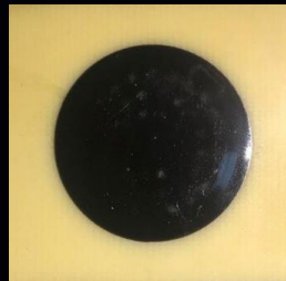
Reinforced solder joint with potting
