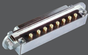
280-052 combo right-angle PC tail pin connector
