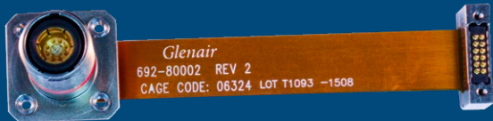
High-speed Glenair cylindrical PCB connector used in a tool segment interconnection flex jumper assembly
