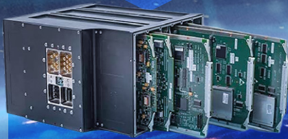
Flight computer with PCIe board-to-board interface
