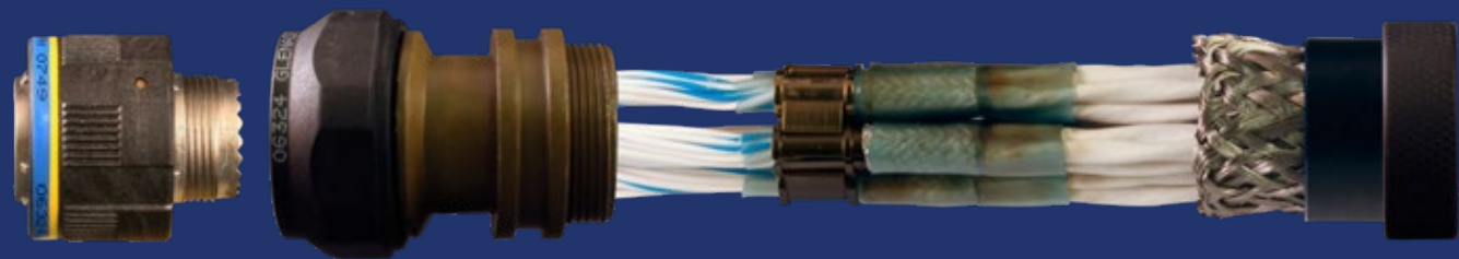
Exploded view of a StarShield assembly termination. Note the use of heat shrink termination material and the Glenair signature StarShield ferrule assembly that results in superior EMC performance compared to conventional individual wire shield termination systems.
