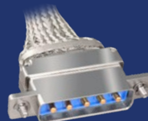
EMI Backshell Adapters These two-piece adapters fit into a groove on Micro-Crimp cable connectors. Attach to connector with screws (provided). Elliptical banding platform provides ample room for large wire bundles.
