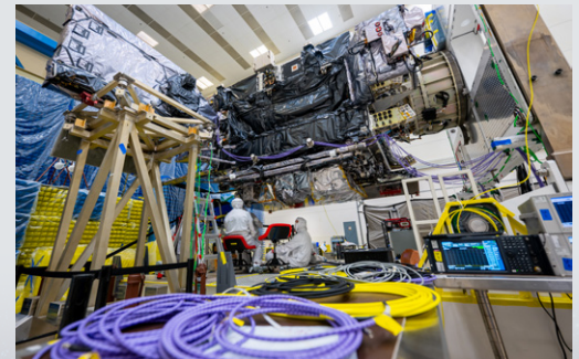
EMI/EMC testing of the NOAA GOES-U satellite
