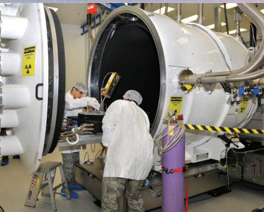
TVAC testing in a USAF environmental test chamber. Glass-sealed hermetic feedthrus maintain enclosure integrity.
