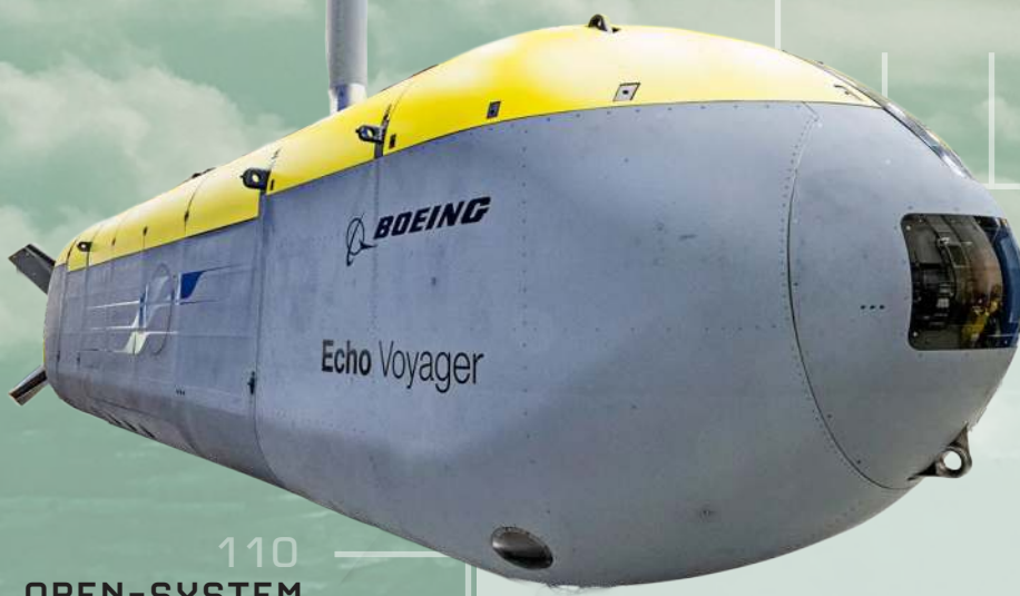
The Boeing XLUV (Extra Large Uncrewed Undersea Vehicle) "Echo Voyager" represents the United States Navy's primary heavy-hitting, long-endurance autonomous submarine program.
