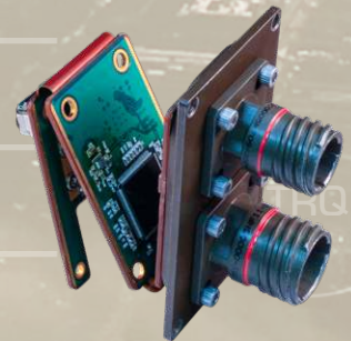
SuperNine Series III embedded PCB assembly with optimized SWaP
