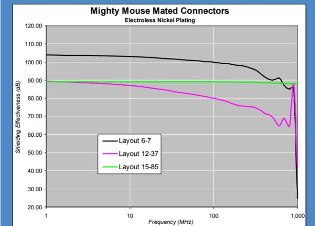
Well designed and engineered connectors will meet the requirements of EIA-364-83 for shell-to-shell conductivity in the initial condition, following salt spray, following 500 mating cycles, and following shock and vibration. In the case of the Series 80 “Mighty Mouse” the mated pair did not exceed the 10 millivolt maximum voltage drop as required under EIA-364-83.
