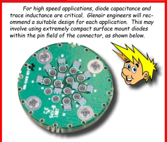
For high speed applications, diode capacitance and trace inductance are critical. Glenair engineers will recommend a suitable design for each application. This may involve using extremely compact surface mount diodes within the pin field of the connector, as shown below.
