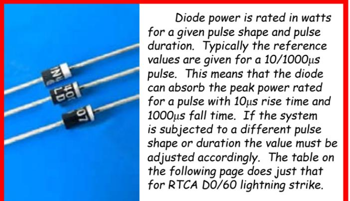
Diode power is rated in watts for a given pulse shape and pulse duration. Typically the reference values are given for a 10/1000µs pulse. This means that the diode can absorb the peak power rated for a pulse with 10µs rise time and 1000µs fall time. If the system is subjected to a different pulse shape or duration the value must be adjusted accordingly. The table on the following page does just that for RTCA DO/60 lightning strike.
