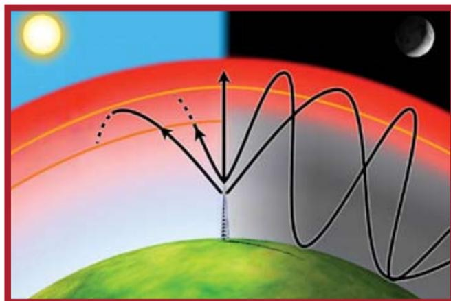
The poster-child of emitted EMI: High-frequency RF wave propagation over long distances—enabled by the unique reflective properties of the ionosphere.
