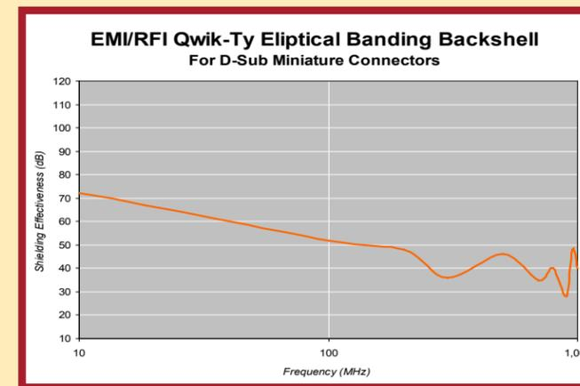
**Shell-to-Shell Conductivity in Mated Connector pairs**
