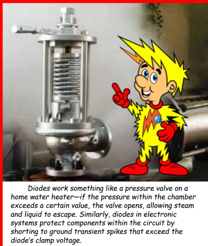
Diodes work something like a pressure valve on a home water heater—if the pressure within the chamber exceeds a certain value, the valve opens, allowing steam and liquid to escape. Similarly, diodes in electronic systems protect components within the circuit by shorting to ground transient spikes that exceed the diode's clamp voltage.
