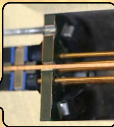
Glenair's state-of-the-art diode burn in process tests leaded and surface mount diodes with leakage current monitored throughout the entire test procedure, ensuring field reliability.
