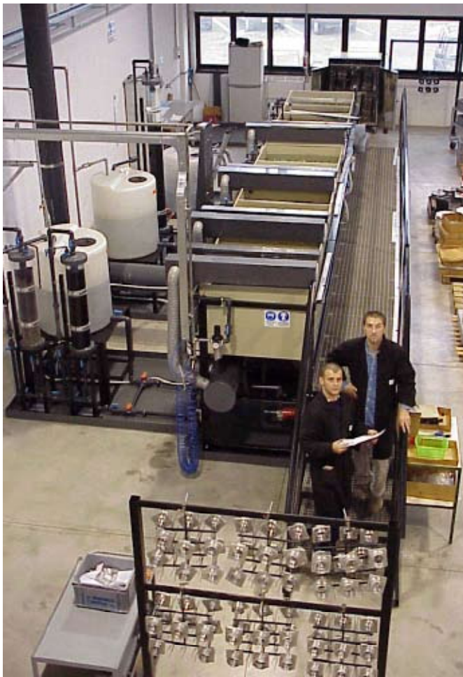
Glenair's electrodeposited paint line is used primarily for commercial grade components, such as our MIL-DTL-5015 (ITS) and MIL-DTL 26482 (IPT-SE) type connector series.
