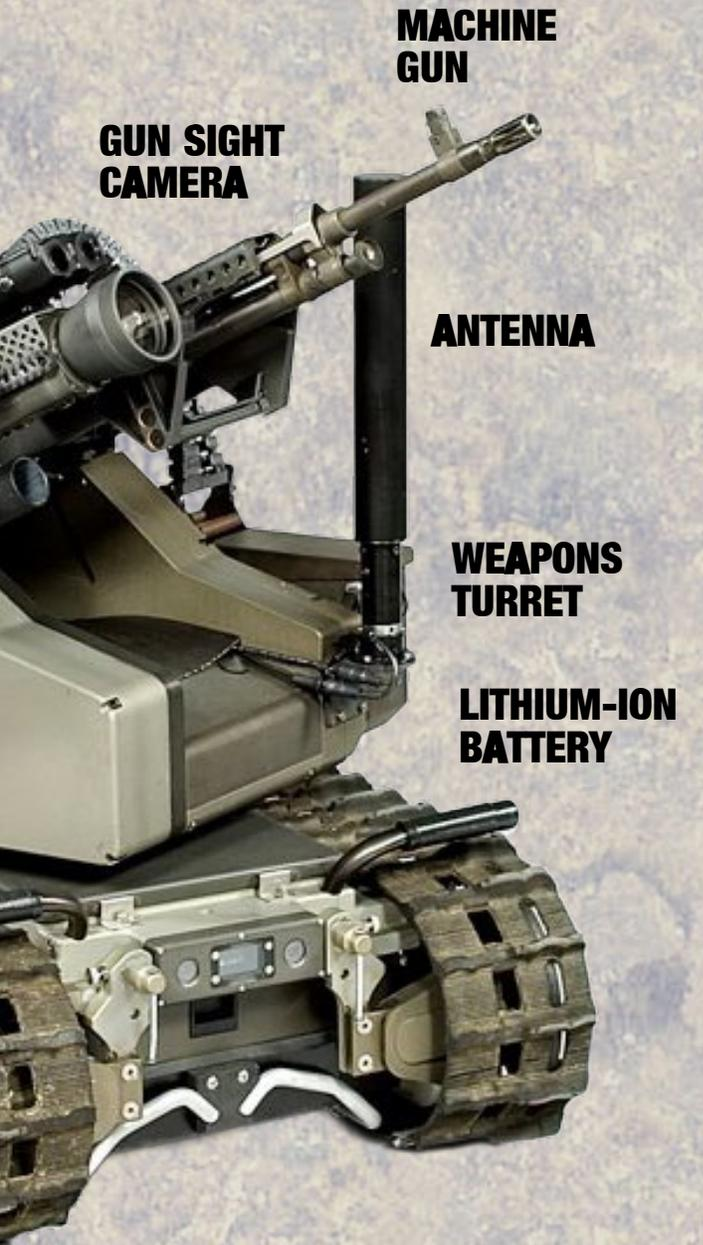
**QinetiQ MAARS non-lethal weaponry includes mounted loudspeakers, high-powered pulsing laser, 40mm non-lethal ammunition (including bean bags, smoke, star clusters and pepper spray). For lethal action, the remote-controlled MAARS can launch 40mm HE grenades or fire its 7.62mm machine gun.**
