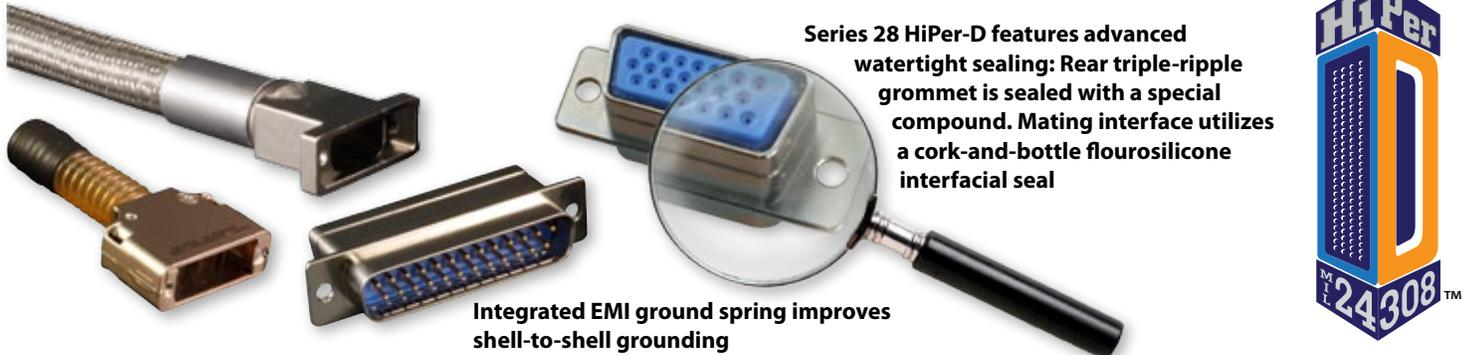
Series 28 HiPer-D features advanced watertight sealing: Rear triple-ripple grommet is sealed with a special compound. Mating interface utilizes a cork-and-bottle flourosilicone interfacial seal
