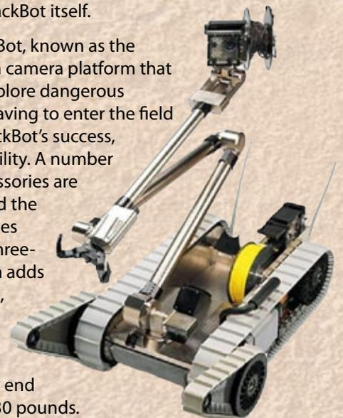
PackBot can also be equipped with a suite of powerful sensors, including additional cameras and laser range-finders. A HazMat unit includes sensors that detect the presence of toxic or radioactive materials, while the EOD (explosive ordnance disposal) version of PackBot can detect, remove or defuse explosives. There's a lighter, higher speed version of PackBot, and even one that can zero in on snipers by acoustically analyzing gun fire.
