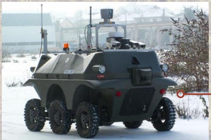
The Thales R-Trooper is a 6X6 wheeled, multipurpose UGV designed for area control, perimeter surveillance, and IED clearance, and can transport multiple small UGVs.
