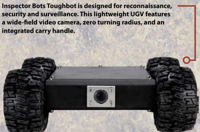
Inspector Bots Toughbot is designed for reconnaissance, security and surveillance. This lightweight UGV features a wide-field video camera, zero turning radius, and an integrated carry handle.
