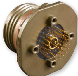
233-218 Jam-Nut Receptacle with hybrid signal and Quadrax contacts, PC tail termination and threaded standoffs for reliable connector-to-board attachment
