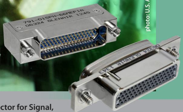
The Series 791 is a The Scoop-Proof High-Performance Environmental Connector for Signal, Power, RF, and Datalinks. It combines the versatility of the Series 790 Micro-D connector with the rugged features of our popular HiPer-D M24308 type connector. High performance features include Scoop-proof pin protection, blind mating, rugged environmental and EMI protection. This space-grade connector is offered in 37 arrangements and 12 machined shell sizes for complete versatility.
