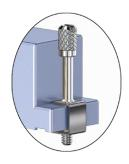
Replacement socket head male screwlock for Type 2 solid Series 557 backshells with .25 (6.4) flange. 300 Series stainless steel.
