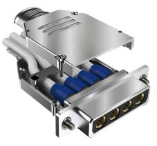
This precision-machined 799-164 nonenvironmental piggyback backshell fits Series 792 connectors. Backshell has internal fluorosilicone wire strain relief grommet optimized for axial alignment and support of twinax, quadrax or octaxial Ethernet cables.
