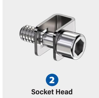
Stainless steel screwlock and jackscrew kits fit Micro-D connectors without backshells. Screwlocks allow the connectors to be fully mated before the screws are tightened. Jackscrews must be tightened in order to mate connectors. Kit consists of (1) screw and (1) retainer clip, *order (2) kits per connector*. Jackscrew and clip are passivated stainless steel.
