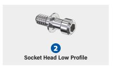
Stainless steel Micro-D jackscrew kits conform to MIL-DTL-83513/05. Kit consists of (2) jackscrews and (2) retainer rings. Choose slotted head or socket head. Two thread sizes: 2-56 for size 9 to 69, 4-40 for sizes 79, 100 and 130. Place jackscrew through connector mounting hole, then slide e-ring into slot on jackscrew.
