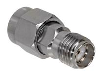
2.92 Male / SMA Female. GRF05-0026 adapter connects 2.92mm female to SMA male. Stainless steel body, coupling nut and lock ring. Gold-plated BeCu contact, PTFE insulator, silicone gasket.
