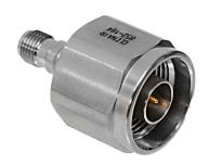
**NMale/SMA Female.** Connect N jack to SMA plug with GRF05-0019 adapter. Stainless steel body with gold-plated BeCu contact, PTFE insulator, nickel-plated phos bronze lock ring, and silicone gasket.
