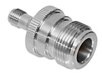
**N Female / SMA Female.** Connect N plug to SMA plug with GRF05-0020 adapter. Stainless steel body, gold-plated BeCu contact, PTFE insulator.
