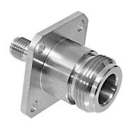
N Female / SMA Female. Connect N plug to SMA plug with GRF05-0022 panel mount adapter. Stainless steel body, gold-plated BeCu contact, PTFE insulator.
