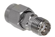
2.92 Male / SMA Female. GRF05-0026 adapter connects 2.92mm female to SMA male. Stainless steel body, coupling nut and lock ring. Gold-plated BeCu contact, PTFE insulator, silicone gasket.
