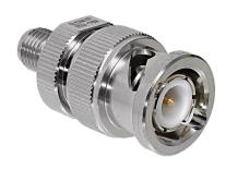
BNC Male / SMA Female. GRF05-0033 adapter connects female BNC to SMA male connector. Stainless steel SMA body, nickel-plated brass BNC body and coupling nut. Gold-plated BeCu contact, PTFE insulator, nickel-plated brass wave washer. Silicone gasket.
