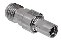
SMP Male / SMA Female. GRF05-0029 adapter has smooth bore SMP male connector interface. Stainless steel body, gold-plated BeCu contact, PTFE insulator.
