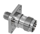
TNC Female / SMA Female. 4 Hole Flange. Connect TNC plug to SMA plug with GRF05-0017 adapter. Stainless steel body, goldplated BeCu contact, PTFE insulator.
