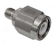
TNC Male / SMA Female. Connect TNC jack to SMA plug with GRF05-0015 adapter. Stainless steel body with gold-plated BeCu contact, PTFE insulator, nickel-plated phos bronze lock ring, and silicone gasket.
