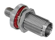
TNC Female / SMA Female. Jam nut panel mounting. Connect TNC plug to SMA plug with GRF05-0018 adapter. Stainless steel body and hex nut. Gold-plated BeCu contact. Nickel-plated brass lock washer, PTFE insulator, silicone O-ring.
