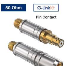
G-LinkRF. SMA adapter. 18 GHz. 50 ohm. Size 8. Snap-in, rear release coax contacts fit Glenair Series 795 and Series 806 RF connectors with size 8 contact cavities. BMB-style contact features G-LinkRF female SMA adapter and integral release sleeve. Attach male SMA plug directly to contact, no soldering required. 50 ohm nominal impedance. DC - 18 GHz frequency range.
