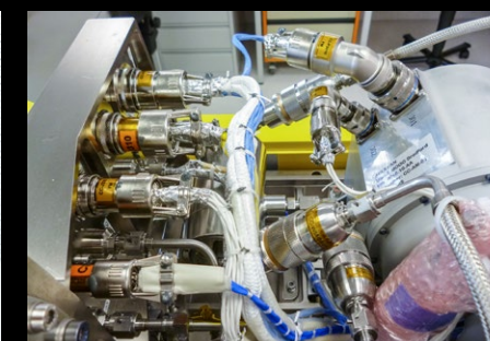
EMI shielded and open-wire bundle assemblies ready for flight
