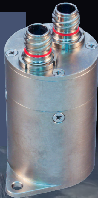
Connectorized HDRM with Mighty Mouse connectors
