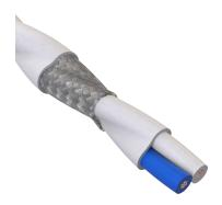
Glenair 963-073-26 protocol-specific cable is designed for high speed data transmission up to 2 GHz with a 100 Ohm differential impedance, making it ideal for avionics, vetronics, and digital network applications. Its broad temperature range of -65°C to +200°C ensures reliable performance in demanding environments, from sensor interconnects to serial buses. With robust construction, it's the perfect choice for critical systems like cabin management, high-density connectors, and LVDS devices.
