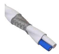
Glenair 963-073-28 protocol-specific cable is designed for high speed data transmission up to 2 GHz with a 100 Ohm differential impedance, making it ideal for avionics, vetronics, and digital network applications. Its broad temperature range of -65°C to +200°C ensures reliable performance in demanding environments, from sensor interconnects to serial buses. With robust construction, it's the perfect choice for critical systems like cabin management, high-density connectors, and LVDS devices.
