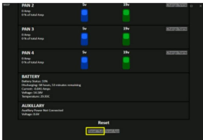
After tapping “Reset Hub” at the bottom of the screen, the user will see the blue and green voltage switches of all the ports reset.
