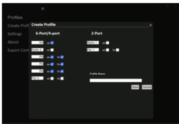
In creating a profile you can set a name for each port. The 5V and/or battery power can also be enabled/disabled for each port. Radio ports only have battery power in.
