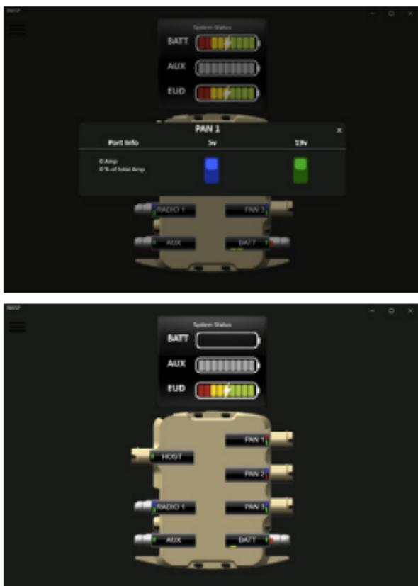
Disable/Enable function allows user to save power by Disabling 5V (blue button) or battery power (green button) supply to peripherals without cutting data communication.
