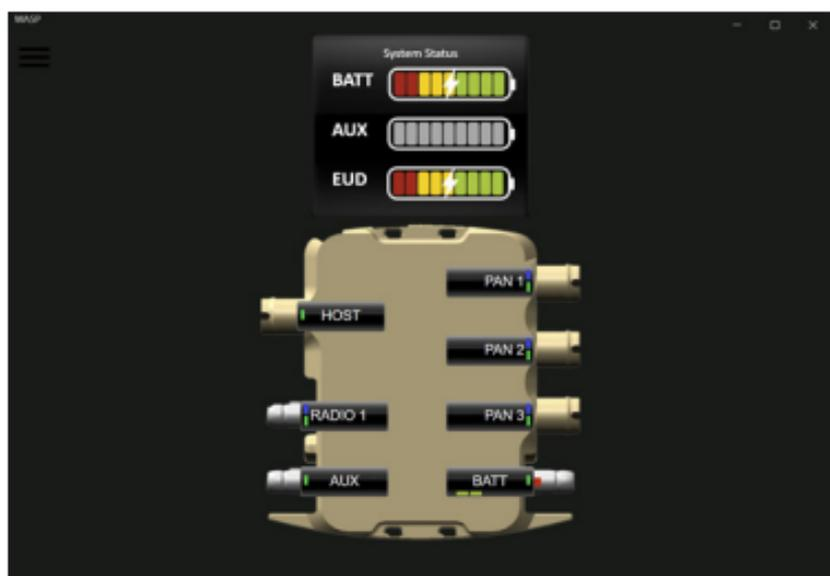
If an auxiliary power supply is connected to the STAR-PAN Hub, it is used by the system to charge the main battery, and individual port devices.
