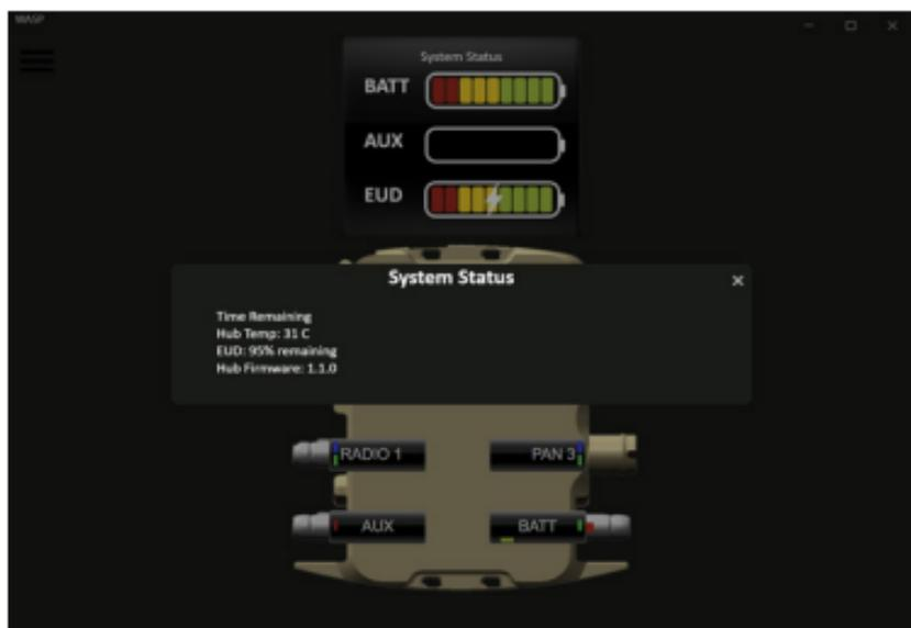
*System status box* will show graphical representation of EUD battery status and status of connected batteries on BATT/AUX port (for all SMBus-compatible batteries).
