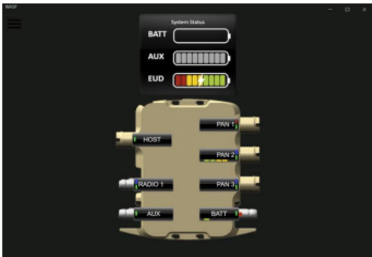
Enabled devices draw power. The amount is shown visually in a power load status bar directly under the port name.
