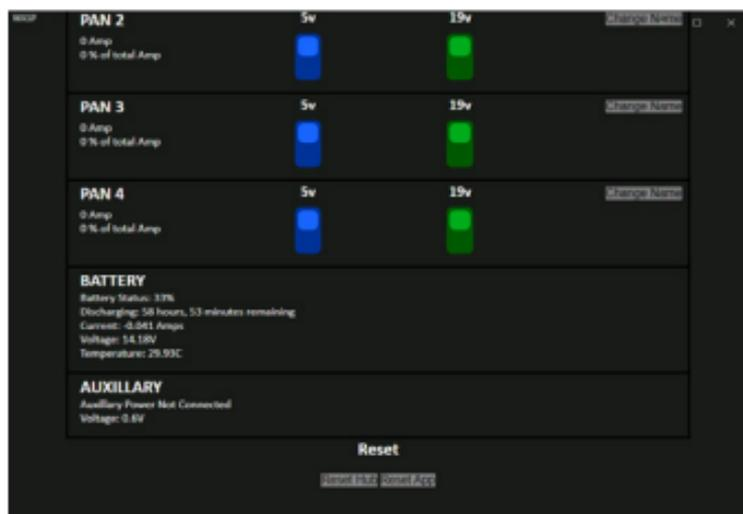
To reset the hub and app, swipe left from the hub screen view. Scroll to the bottom of the list screen view. This is where the 'Reset' options are.
