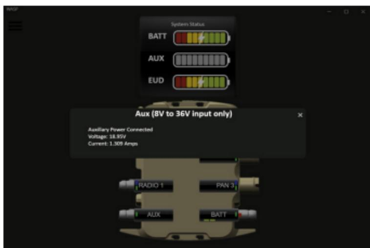
If the AUX power port is plugged to an AC power supply, the AUX power status bar will appear light gray. Click/tap on the AUX port to display input voltage and current.
