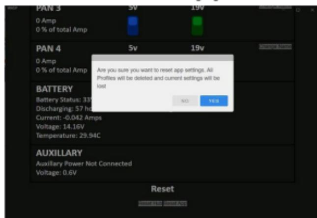
Upon tapping “Reset App Defaults” from the menu options screen, a pop-up alert confirming to clear all profiles, reset the hub, and return the system to factory defaults will appear. Select “Yes” to wipe all saved information and reset the hub.
