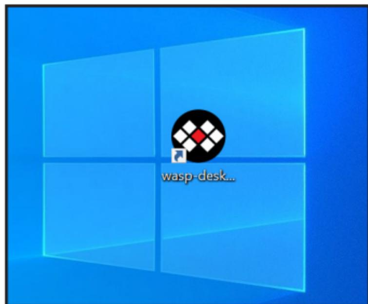
Once connected, the EUD Host will recognize the STAR-PAN IV connection. Double-click the WASP icon to launch the application.
