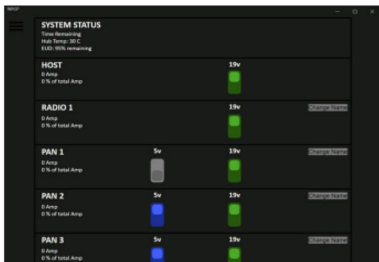
Slide left from the main screen to view a second port-status “home screen” lists that details battery power usages stats for all devices on the system. Note that you will only receive SMBus data if connected to a smart battery
