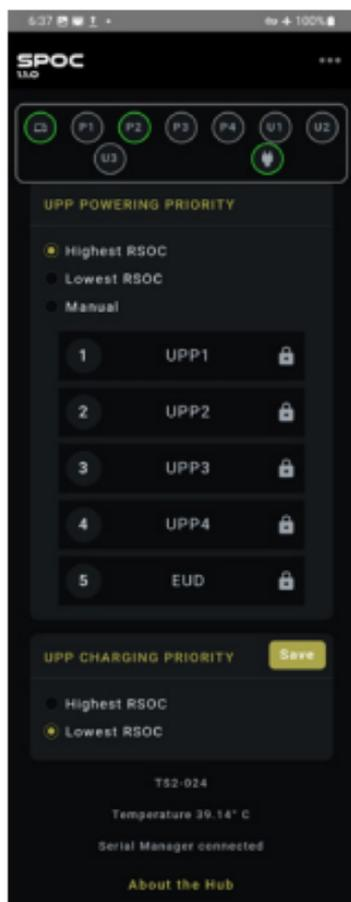
**UPP Charging Priority** is used to determine which battery will be charged when multiple batteries are connected at the same time as a Power Supply. Only one battery is charged at a time. Charging selection is determined every time a power source is connected/disconnected or a battery is fully charged.
