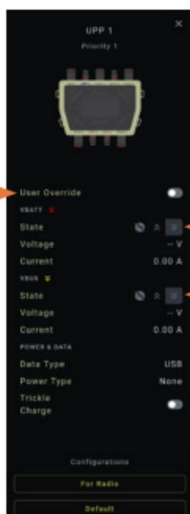
VBATT and VBus can be set to input, output or disabled.
