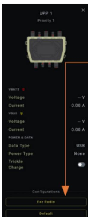
Select the "For Radio" button to configure the UPP as a legacy Radio Port
