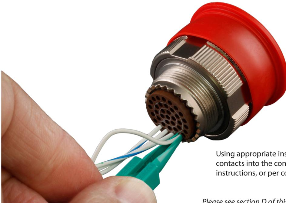
Using appropriate insertion tools, insert terminated contacts into the connector per Glenair insertion instructions, or per connector manufacturer's procedure.
