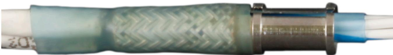
Be careful not to overheat preform assembly and scorch outer shrink sleeve. Slight browning of outer shrink sleeve is acceptable, but severe discoloration is indicative of improper termination.
