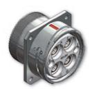
921-003 Rear panel mount, wall mount receptacles feature EMI protection through the use of a ground spring. Accessory threads for backshells with integral teeth for high vibration environments. Clinch nuts eliminate the need for tapping mounting holes or nut. Optional gold-plated signal (Size 16 and 12) contacts available for improved corrosion protection in space or petrochemical environments. Silicone O-rings and wire seal provide watertight sealing. Contacts are included.
