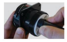
11. To remove the contact use the removal tool (see the "Insertion and Removal Tool" table on page G-6). Insert the tool from the front end of the connector and push it over the contact thoroughly. At the same time pull the cable from the rear end.
