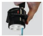
**8.** Insert the contact from the rear side. Push the cable until a click of the internal locking clip can be felt.
