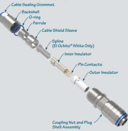
Cable connectors feature gold-plated crimp contacts, precision insulators, integral backshell, sealing grommet and machined shells. Cable connectors are available as unassembled kits or ready-to-use factory-terminated cordsets.
