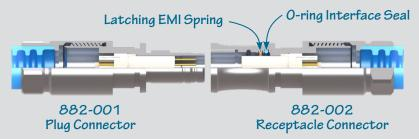
Push-pull SuperFly Datalink receptacle connectors feature a canted coil spring for secure mating and excellent EMI protection. A fluorosilicone O-ring provides watertight sealing when mated.
