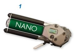
The 601-108 Nano Band-Master™ ATS Tool weighs 1.18 lbs., and is designed for nano flat .075" width clamping bands (601-500, 601-504 and 601-508) in a tension range from 20 to 50 lbs. Calibrate at 50 lbs. ± 3 lbs. for most shield terminations. Tool and band should never be lubricated.
