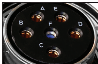
Cavity F contains a Pitot tube Socket contact
