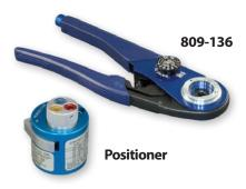
**809-136** Crimp tool for use with size #20, #16 and #12 power pins. 9.75 inches OAL, 1.25 pounds. Use with M39029/57 and /58 contacts and 809-093 adapters.
