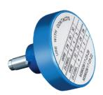
Positioners for use with 809-015 miniature adjustable crimp tool. These bayonet-type positioners hold contacts at correct height for crimping with M22520/2 type miniature step adjustable tools, above. Face plate shows correct tool settings.
