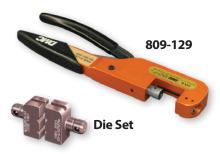
**809-129** Parallel action tool for use with hex crimp dies. 11 inches OAL, 2.0 pounds. Anodized aluminum frame, steel mechanism, plastic handles. Includes tool for die set extraction. Accepts all M22520/5 die sets.
