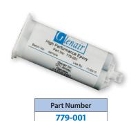
High performance flexible two part thermoset epoxy provides high strength flexible bond from -55° to 150°C. 50 ml duo syringe fits standard dispensing guns. Use with square green mixing nozzle sold separately. 12 hour cure time at 20°C, 1 hour at 85°C, 30 minutes at 150°C. Apply to inside of boot with wooden spatula. 18 month shelf life.
