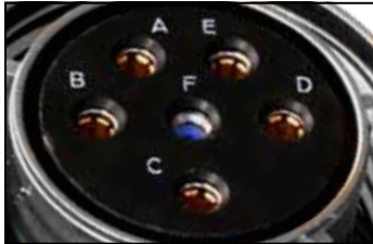
Cavity F contains a Pitot tube Socket contact
