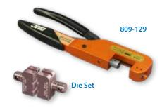
**809-129** Parallel action tool for use with hex crimp dies. 11 inches OAL, 2.0 pounds. Anodized aluminum frame, steel mechanism, plastic handles. Includes tool for die set extraction. Accepts all M22520/5 die sets.
