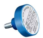
Positioners for use with 809-015 miniature adjustable crimp tool. These bayonet-type positioners hold contacts at correct height for crimping with M22520/2 type miniature step adjustable tools, above. Face plate shows correct tool settings.
