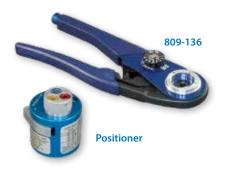
**809-136** Crimp tool for use with size #20, #16 and #12 power pins. 9.75 inches OAL, 1.25 pounds. Use with M39029/57 and /58 contacts and 809-093 adapters.
