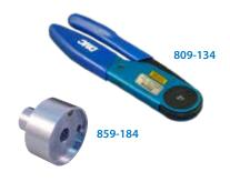
809-134 crimp tool for size #8 el Ochito® 858-028-02 round crimp shield sleeves. Tool features ratchet mechanism to prevent damage from over crimping. Check calibration with G426 gage.
