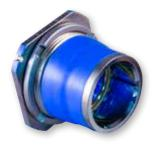
Float mounting: allows for a modicum of coplanar movement of the receptacle during rack-and-panel and other blind mate applications, preventing both contact and shell damage.
