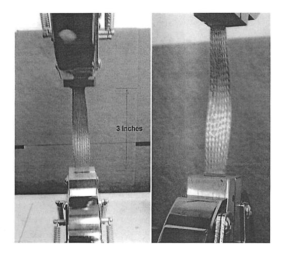
Part 5: Calibrate the Instron by zeroing out the display's force reading without braid being pulled (braid shall be relaxed).
