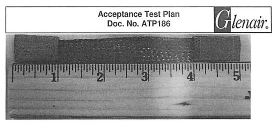
Part 4: Place the sample between the wedge action grips and make sure the action grips are tight enough. Make sure the three (3) inches of the braid is visible.
