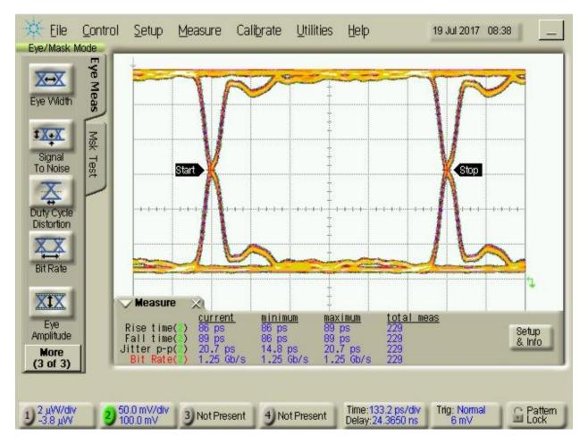
Figure 3: Eye diagram of GSGSG configuration at 1.25Gbps
