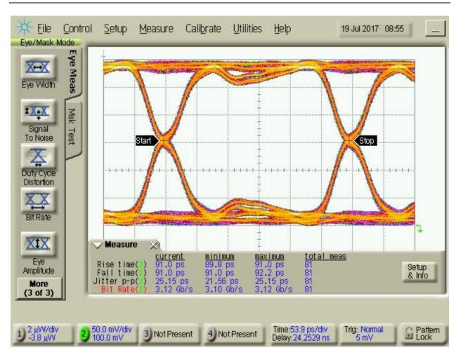
Figure 12: Eye diagram of DGSSG configuration at 3.125Gbps
