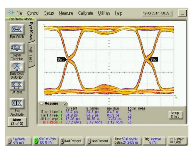
Figure 4: Eye diagram of GSGSG configuration at 3.125Gbps
