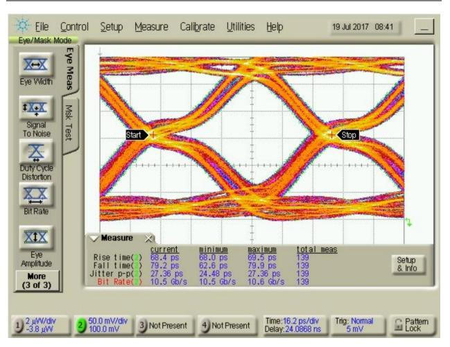
Figure 6: Eye diagram of GSGSG configuration at 10.3125Gbps
