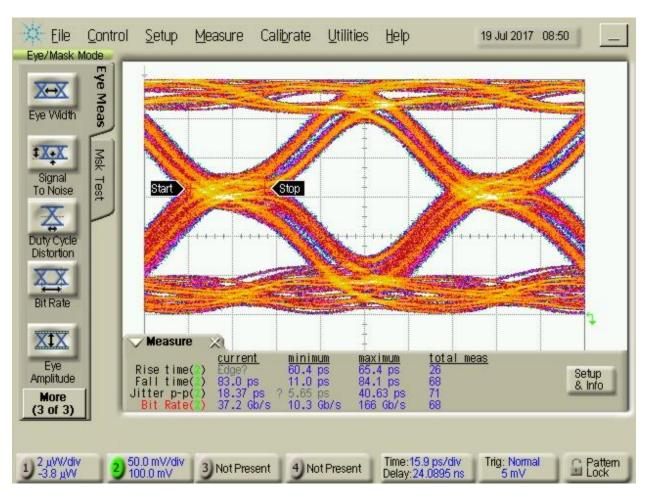
Figure 10: Eye diagram of GSSG configuration at 10.3125Gbps
