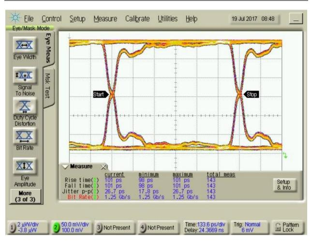
Figure 7: Eye diagram of GSSG configuration at 1.25Gbps
