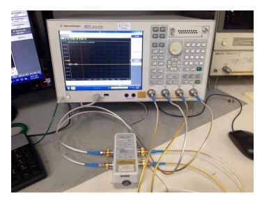
Figure 4: Network analyzer with eCal module
