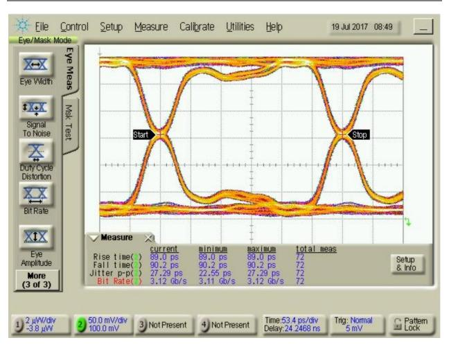
Figure 8: Eye diagram of GSSG configuration at 3.125Gbps
