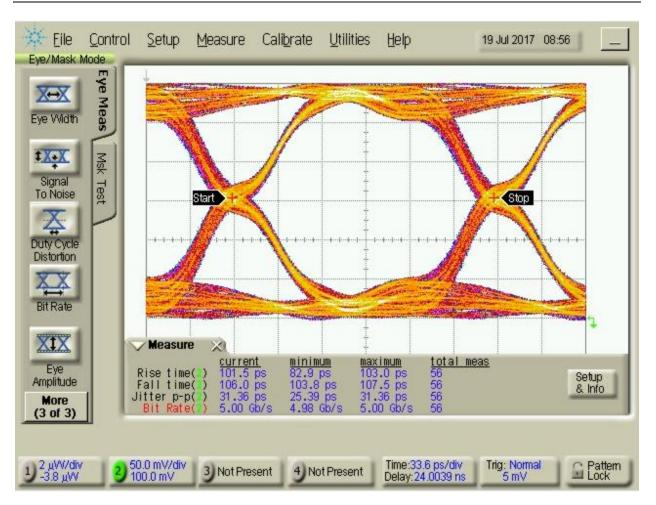
Figure 13: Eye diagram of DGSSG configuration at 5Gbps
