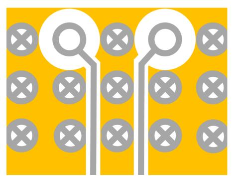
Figure D3. Inner Row Escape Routing
