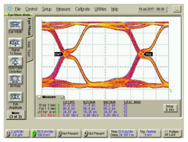
Figure 5: Eye diagram of GSGSG configuration at 5Gbps
