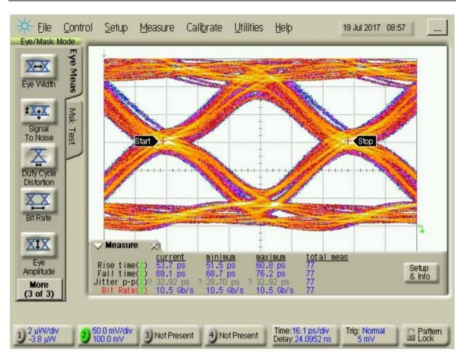
Figure 14: Eye diagram of DGSSG configuration at 10.3125Gbps
