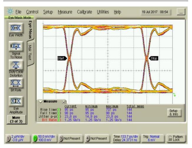
Figure 11: Eye diagram of DGSSG configuration at 1.25Gbps
