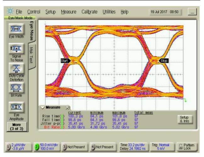
Figure 9: Eye diagram of GSSG configuration at 5Gbps
