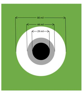
Figure D2. HD Stacker PCB Pad Geometry
