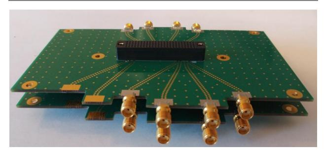
Figure 2. Stacked Test PCBs
