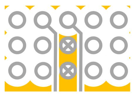
Figure D4. Alternate Inner Row Escape Routing
