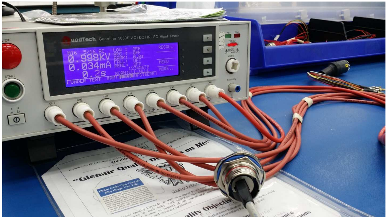
Figure 3. DWV/IR test setup
