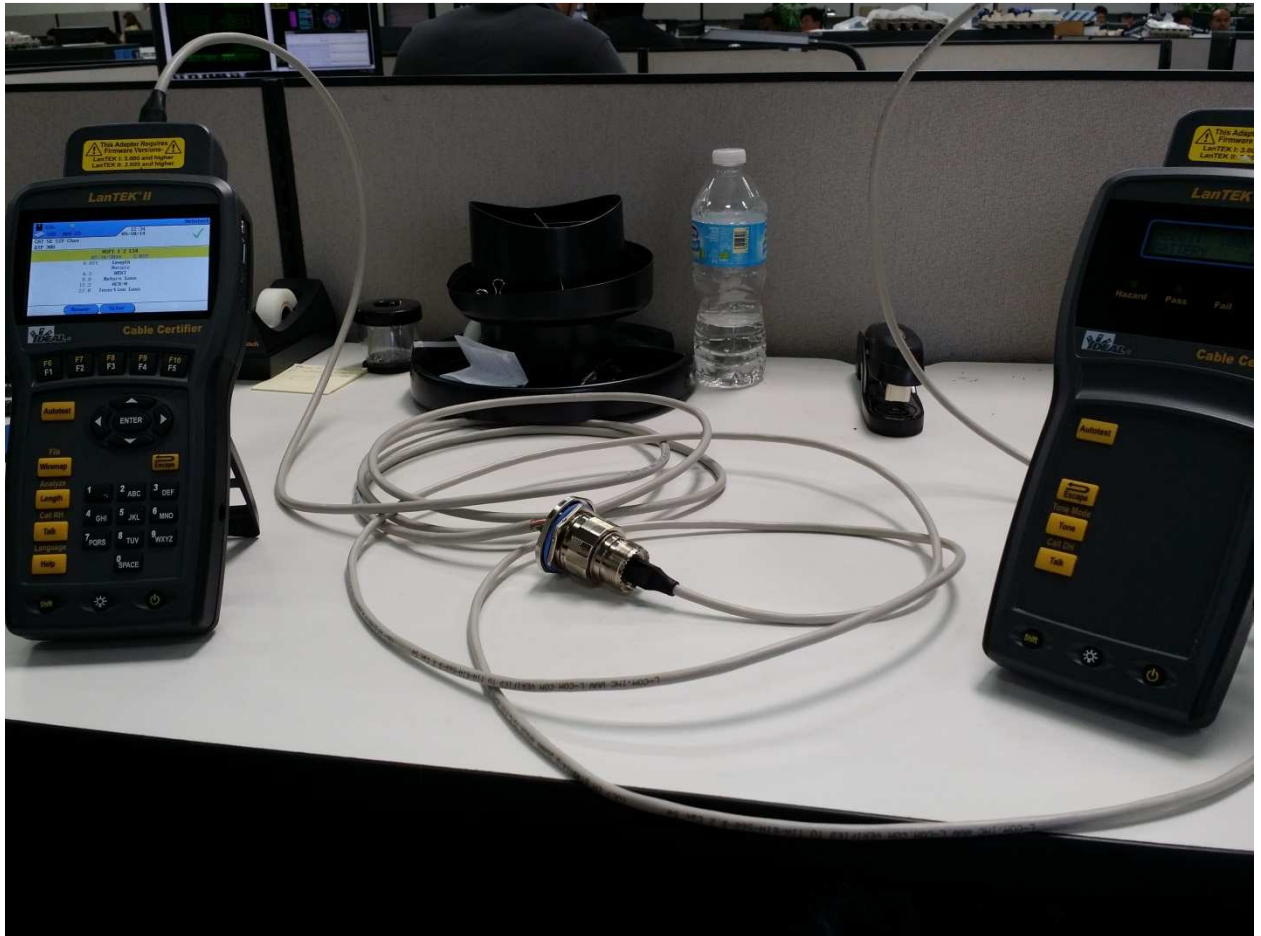
Figure 5. Ethernet Compliance Test.
